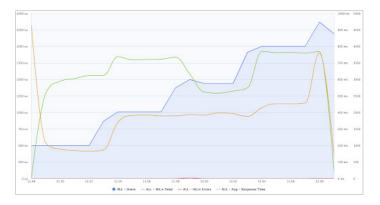
According to New Relic APM, web transaction time is normally at 250 ms. During the load test, web transaction time spiked up to 1,300 ms per request with most of the processing time coming from PHP and Memcached. This would be an area to dive into deeper.
